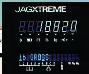
JAGXTREME Terminal: A two-line display shows weights and provides prompts and options for setup.
